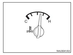
Your vehicle is equipped with an engine coolant temperature gauge. With the ignition in the ON position, this gauge shows the engine coolant temperature.
